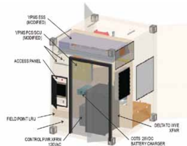
Figure 1 - Mature components. The IEM, illustrated above, uses proven components (such as the ESS) that have been used on BAE Systems' successful hybrid bus programmes.
